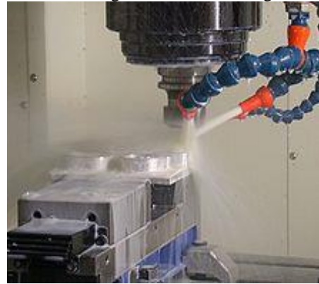
Fig. 5. Vertical Machining Centre – Metal Cutting Operation using emulsified coolant
